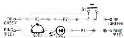
FIG. 2—PARTS-PLACEMENT DIAGRAM. You can make a PC board from the foil pattern we've provided and mount the parts as shown here, or use perforated construction board with point-to-point wiring.
