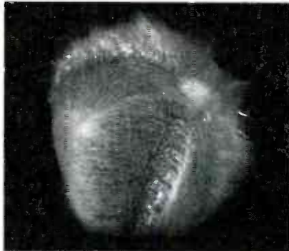
FIG. 8—WATER-FILLED BALLOON hit by a pellet. The sound sensor was used with the report of the gun providing the event trigger.
