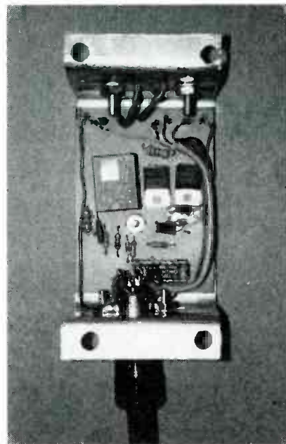
FIG. 5—THE POWER-CONTROLLER board is mounted on a 0.064-inch aluminum plate bent into a U-shaped frame. The DIN socket and the terminal strip are mounted on the sides of the U-bracket.
