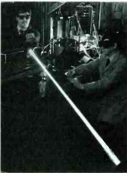
GE SCIENTISTS HAVE GENERATED A 52-WATT GREEN LASER BEAM, more than doubling the previously published brightness record for this wavelength of light produced with solid-state lasers.
