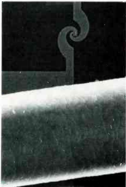
TINY INFRARED ANTENNA developed by NIST scientists is shown next to a human hair.
