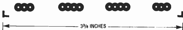
THE FOIL PATTERN OF THE voltage-tripler PC board in the negative ion generator.
