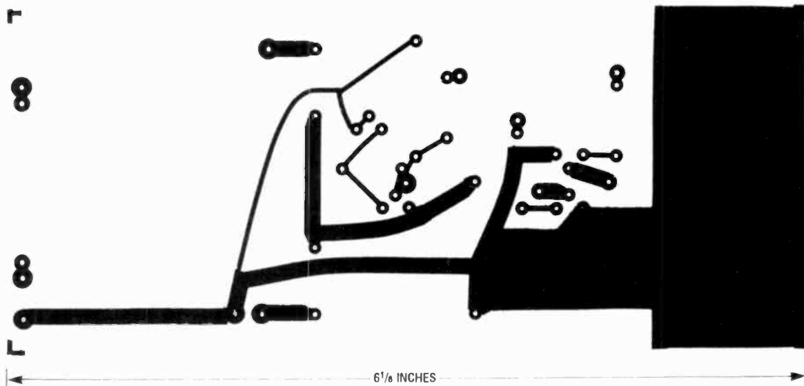
THE FOIL PATTERN OF THE main PC board in the negative ion generator.
