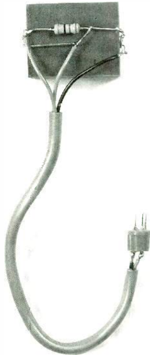
PROTOTYPE VERSION of the simulated laser diode. A hole drilled in the block provides a light path.
