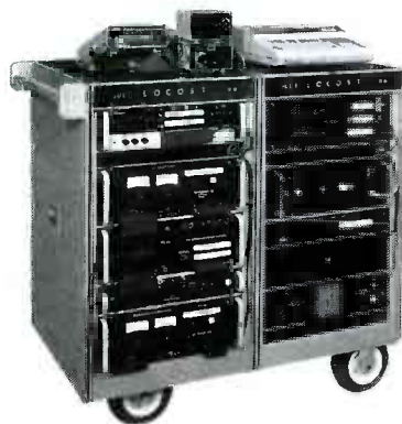
FIG.6—THE JULIE RESEARCH LABORATORIES LOCOST 106. This version automatically calibrates test equipment and calibration standards. The desktop-computer controller is at top right.
