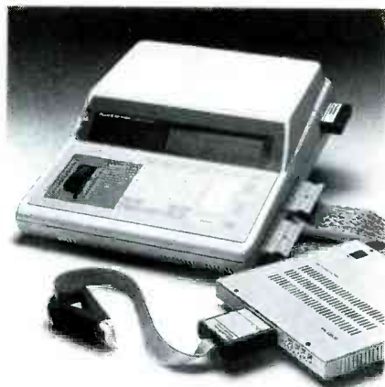
FIG.5—THE FLUKE 900 DYNAMIC TROUBLESHOOTER uses comparison testing as a low-cost alternative to isolate faults to the component level without programming or knowledge of a board. The 900 captures timing errors, intermittent faults, and static device failures, and performs dynamic ICT tests on each IC while operating.
