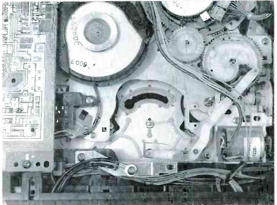
FIG. 4—A TYPICAL LOAD MOTOR is located on the bottom side of the VCR's chassis.
