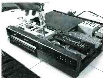
FIG. 2—THE CASSETTE CARRIAGE assembly is usually secured to the VCR chassis by four Phillips-head screws.
