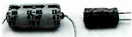
FIG. 3—THE LEADS of an axial-lead capacitor (left) extend along its axis; those of a radial-lead one (right) align with a radius.
