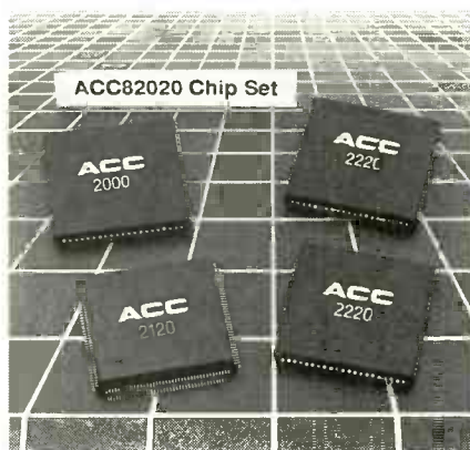
Fig. 1. TURBO PC/AT CHIP SET offers a complete logic complement to 286 and 386SX personal computers. It features 4-way page interleaved memory controller, 16-MHz system clock with zero wait state, and supports LIM/EMS 4.0 protocol/hardware standard.
