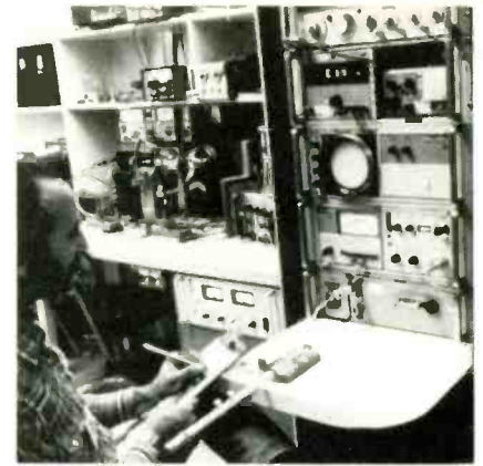
FIG. 7—RF POWER TRANSISTOR IMPEDANCES are determined by measuring the characteristics of a working circuit.
