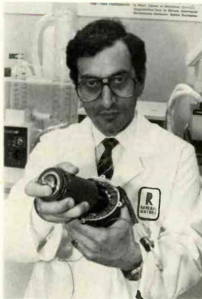
THE MAGNAQUENCH MOTOR to be used in the solar-powered car is unusually small. Dr. Nady Boules, section manager at GMRL's Electrical and Electronics Engineering Dept., is holding the motor's rotor in his right hand, and the motor housing in his left.
