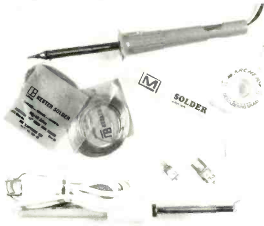
FIG. 1—SMC's CAN BE HAND SOLDERED using only the common tools and materials shown here.
