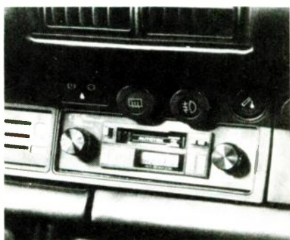
FIG. 7—A CD INPUT and Dolby-C noise reduction are two of the advantages offered by the Autotek SR500.
