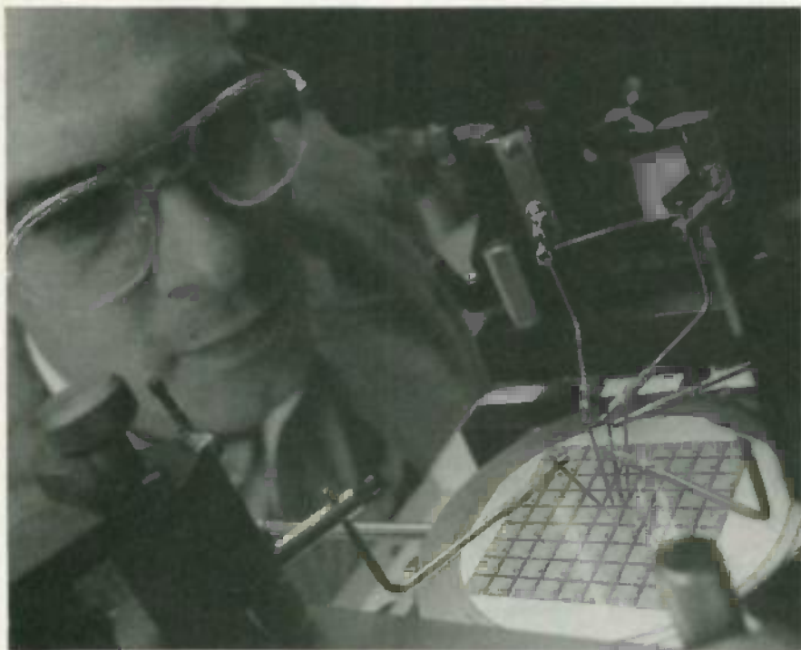
A WAFER OF INSULATED gate transistor power switches about to be tested by G.E. scientist Dr. Eric Wildi. The new devices are so designed that it may be possible to build them right into high-voltage integrated circuits, making it possible for such high-voltage IC's to handle ten times as much power as they do now.
