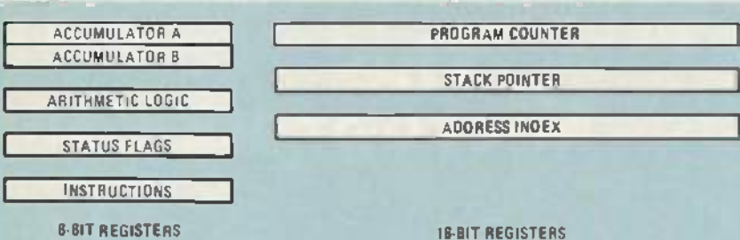
FIG. 3—MOTOROLA'S 6800 emphasizes quick memory access at the expense of few internal registers.
