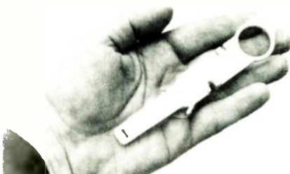
FIG. 17—STRIPPING MODULAR TELEPHONE cable is made much easier with this simple tool. Similar tools are available from a number of suppliers.
