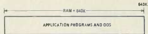
FIG. 4A—IN AN IBM-COMPATIBLE COMPUTER the applications program always attempts to utilize all memory to the highest possible address.
