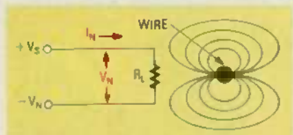
FIG. 3—FIELD-TO-CABLE COUPLING. If a circuit is placed within a time-varying electromagnetic field (such as that generated by a current carrying wire), the field will induce a current and voltage in that circuit.
