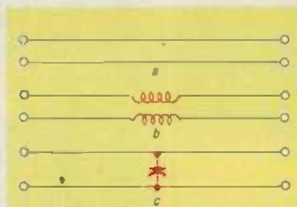
FIG. 4—CABLE-TO-CABLE COUPLING can occur via either inductive coupling (b) or capacitive coupling (c).
