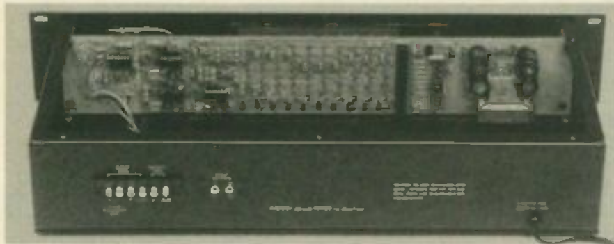
FIG. 7—THE COMPLETED ANALYZER, mounted in a 19-inch rack cabinet. Since most of the components are mounted on the circuit board, there is a lot of room inside the cabinet.
