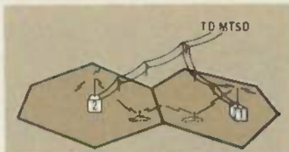
FIG. 3—CELLULAR HAND-OFF occurs as a car moves from cell to cell. During the transfer, which is coordinated by equipment in the MTSO, the user sees no apparent change in transmission quality.
