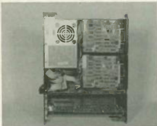
FIG.5—OUR MINIMAL DO-IT-OURSELVES configuration before further upgrading. The disk drives have been installed, along with the disk controller and graphics/monitor adapter boards. Both parallel and serial modules are installed on the disk controller card, which now provides four functions in a single slot. What appears to be a rat's nest of ribbon wire from the parallel and serial modules is just fine; don't try for neatness—Just position the wire wherever it will fit.
