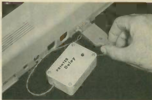
FIG. 7—THE ADAPTER WIRE SLIPS ONTO the computer's Datasette then onto the adapter.
