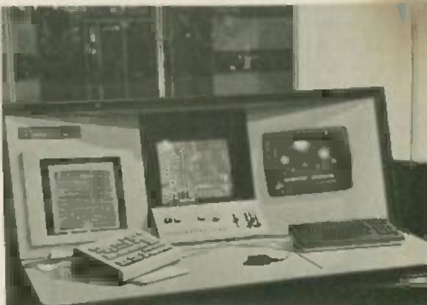
CAD FOR PCB'S: Workstation for Insight , a computer circuit board design system by Scitex Corporation (Israel). Drawn, photographed or digitized artwork can be entered, along with drilling information. The computer enhances the design, checks for errors and draws the finished pattern on its laser scanner.
