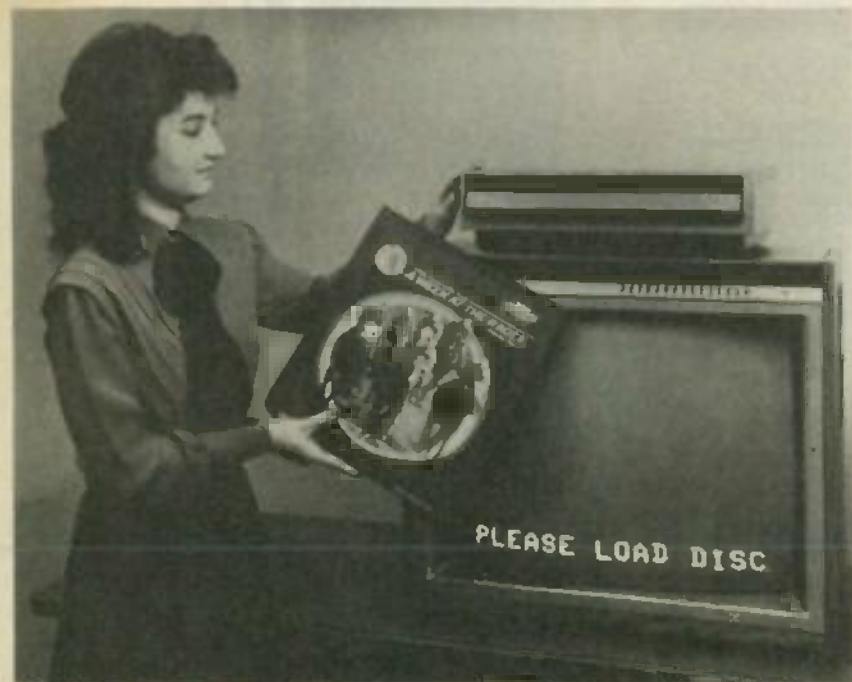
A NEW RCA DEVICE generates TV captions for videodisc and tape players, giving viewers instructions on use, prompting, and timing of the player.
