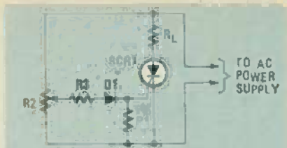
FIG. 8—THE CONDUCTION PERIOD of the SCR can be varied by changing the setting of R2.
