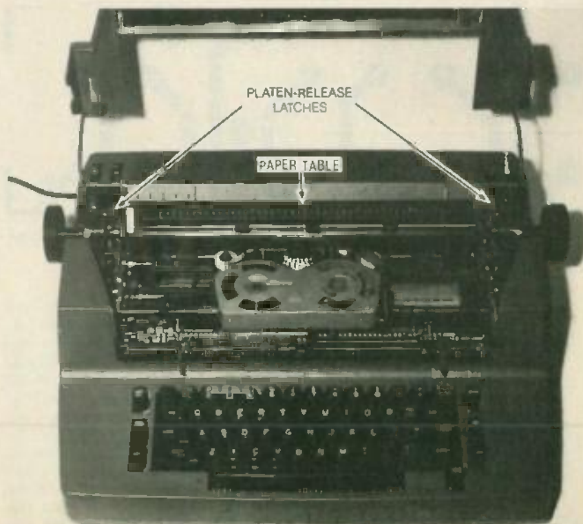
FIG. 16—TO REMOVE THE COVER of the Selectric model II or III, you first must remove the platen.
