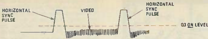
FIG. 4—THE OUTPUT OF IC1 (pin 5) should have a minimum amount of video between the sync pulses.
