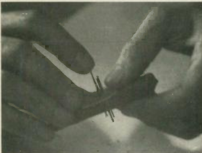
FIG. 3—YOU NEED A PIECE of perforated construction board, about one inch square, to use as a template for electrode spacing.
