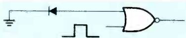
FIG. 7—A DIODE IS USED to imitate a "high" input for an ECL gate.
