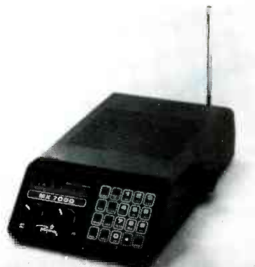
FIG. 13—THE REGENCY MX 7000 offers continuous coverage from 27-1250 MHz.
