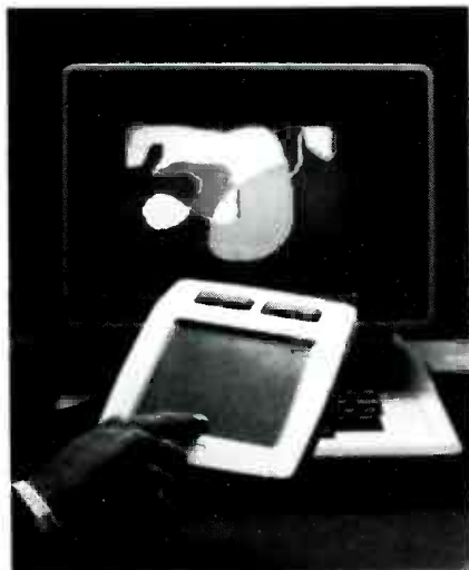
FIG. 7—THE KOALAPAD , from Koala Technologies Inc., is a low-cost touch panel for use with microcomputers.
