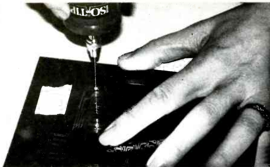
FIG. 15—IF THE BOARD IS DOUBLE SIDED, tape one of the negatives to the board and drill out four of the feedthrough holes. Those holes will be used later to make sure that the two sides of the board are in register.
