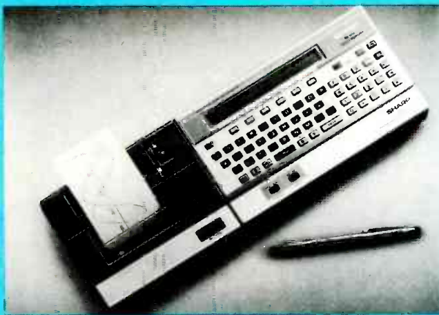
THE SHARP PC-1500 uses an eight-bit CPU. It is shown here with its optional four-color printer/plotter.
