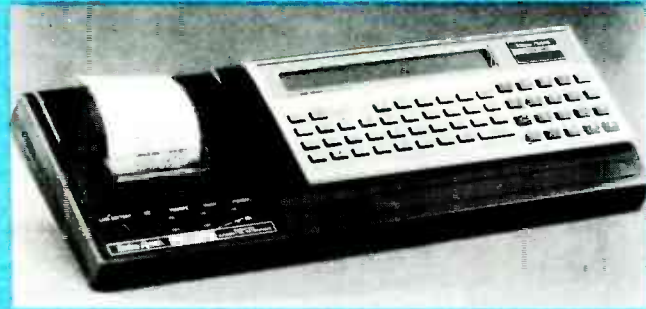
THE RADIO SHACK TRS-80 Pocket Computer uses two, four-bit, micro-processors.
