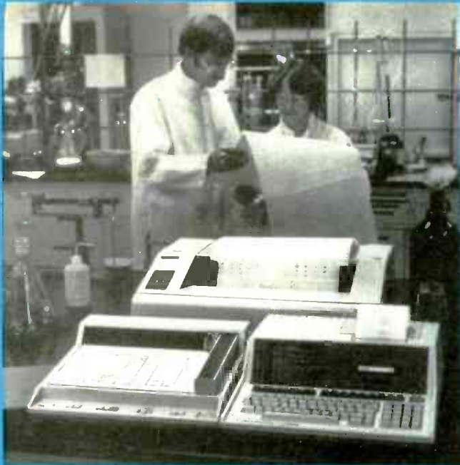
A POWERFUL COMPUTER IN ITS BASIC FORM, the power of an HP-85 from Hewlett-Packard can be increased with the addition of a printer and plotter.
