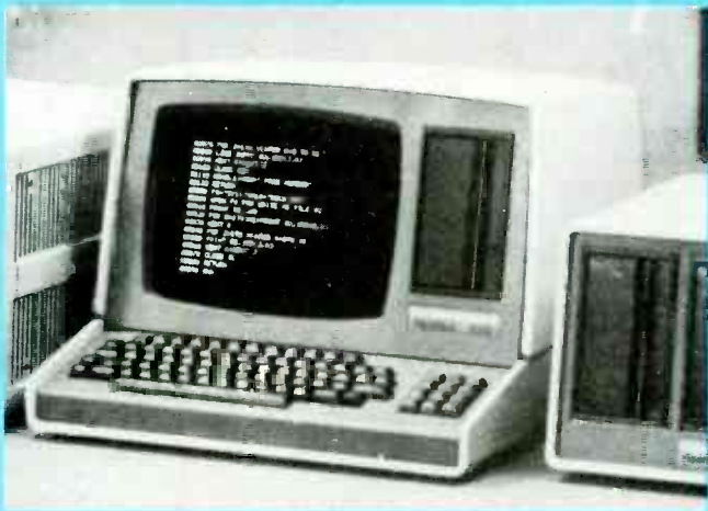
THE ZENITH Z90 is an upgrade of the Z89. The terminal-type housing looks identical for both computers.
