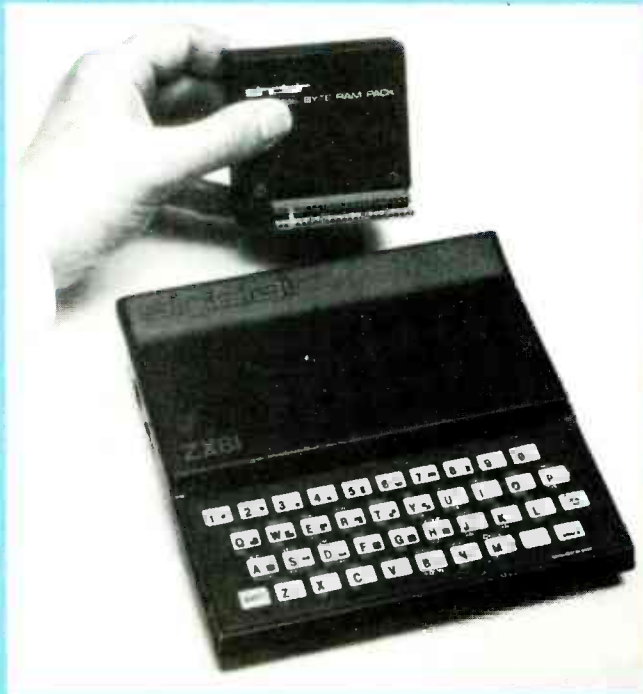
THE MEMORY CAPACITY, and the sophistication, of the Sinclair ZX81 can be increased by adding a 16K memory-expansion module.
