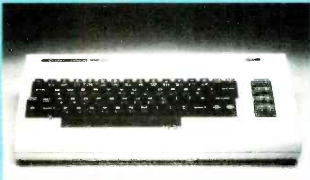
ANOTHER INEXPENSIVE MACHINE from Commodore, the VIC 20's memory can be expanded to 32K.
