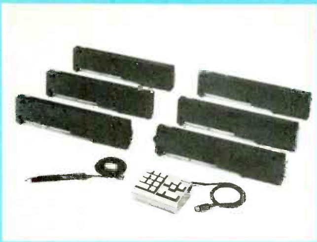
EXPANSION MODULES for the Sony SMC-70. Along with the modules, the light pen and numeric keypad are shown.
