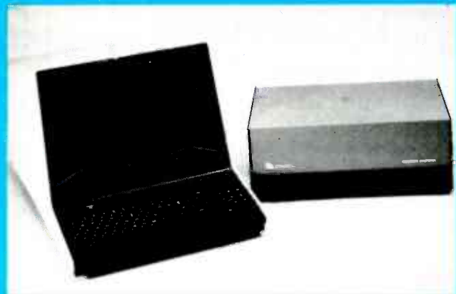
IN ITS NEARLY FULLY CONFIGURED FORM, the Netronics Explorer 85 includes a floppy-disk drive and CP/M.
