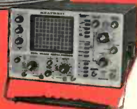
DC-35 MHz dual-trace delayed-sweep oscilloscope
