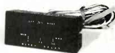
FIG. 6—WIPER CONTROL from Sears works only when the car's wiper switch is off.
