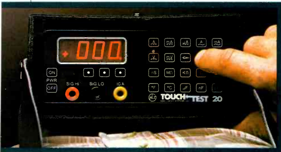
The new Touch Test 20 DMM weighs only 2 lbs. 4 oz. Yet it puts twenty key test functions at your fingertips. Plus exclusive light pressure touch function selection. Shown from above on leather shoulder sling (optional).
