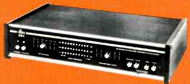
THE MODEL 3BX from dbx is a three band expander that also serves as a noise reduction unit.
