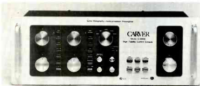
THE MODEL C-4000 preamp from Carver uses only a moderate amount of noise reduction (8 dB) to minimize audible side effects.
