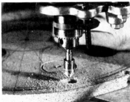
FIG. 30—COUNTERSINKING holes in the bulkhead prevents screwheads from protruding.
