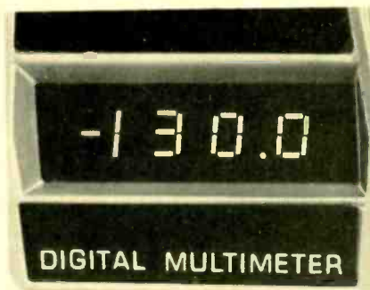
TYPICAL LED DISPLAY is easier to read than LCD display but it consumes more power.
