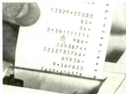
The direct-impression dual discs print cleaner and sharper on conventional paper tape.
