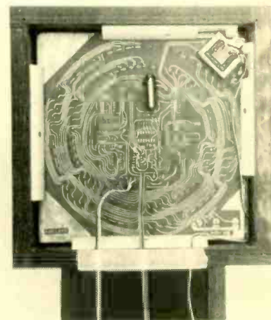
AMELECT CL-7402 time-display circuit board.
