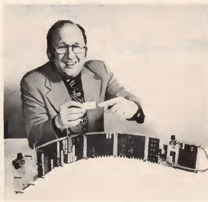
PROTOTYPE of Omega system is 4-foot long and contains over 400 standard IC's.
