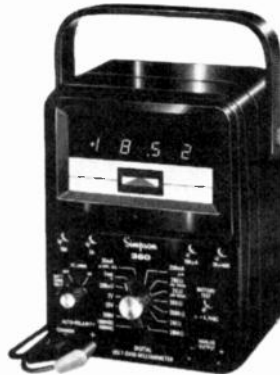
FIG. 19—SON OF 260 is the Simpson model 360 digital vom.
