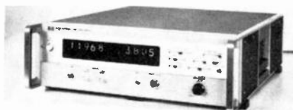
FIG. 12—AUTOMATIC CAPACITANCE BRIDGE has a dual digital readout.
