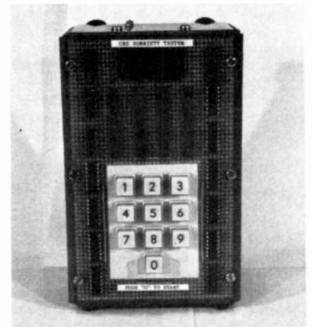
FIG. 21—MOST UNUSUAL DIGITAL instrument we found is this Green Bank Scientific Sobriety Tester.
