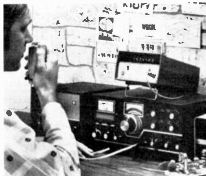
FIG. 7—A FREQUENCY COUNTER can be used to check the frequency of an amateur radio rig.
