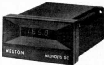
FIG. 4—A SINGLE IC does all the work in this digital panel meter.
