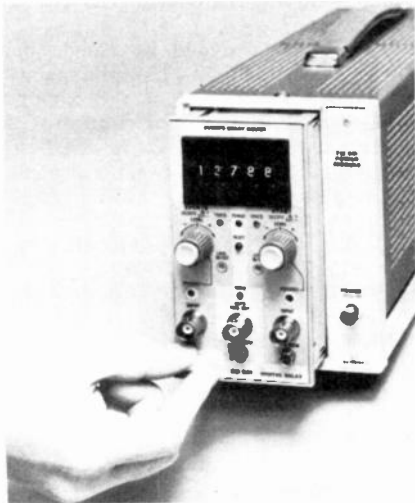
FIG. 17—DIGITAL DELAY MODULE by Tektronix. Thumbwheel switch for getting count is also digital readout.
