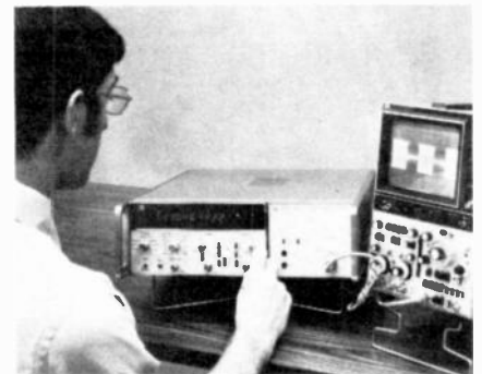
FIG. 8—HIGH-FREQUENCY MEASUREMENTS can be made with instruments like H-P 5354A. It goes to 4 GHz.
