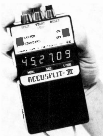
FIG. 13—ELECTRONIC STOP WATCH by TAFCO is a different kind of digital instrument.
