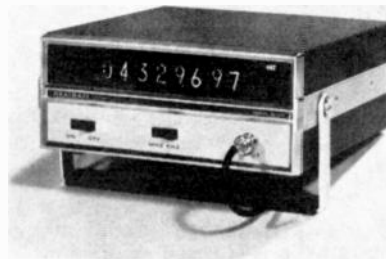
FIG. 6—THIS FREQUENCY COUNTER has eight digits in its readout and goes out to 120 MHz.
