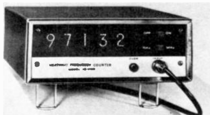
FIG. 5—HEATHKIT MODEL IB-1100 frequency counter uses Nixie type readout.
