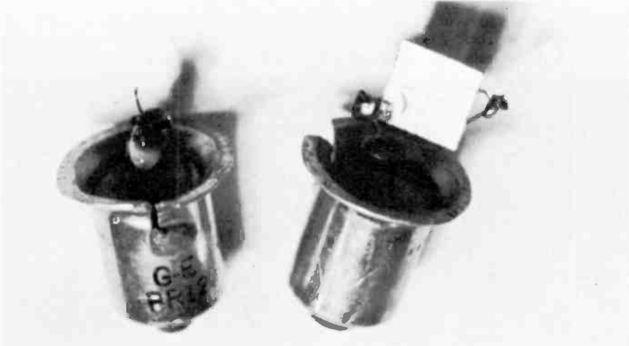
TWO TYPES OF DETECTORS can be mounted equally well on the lamp base.
