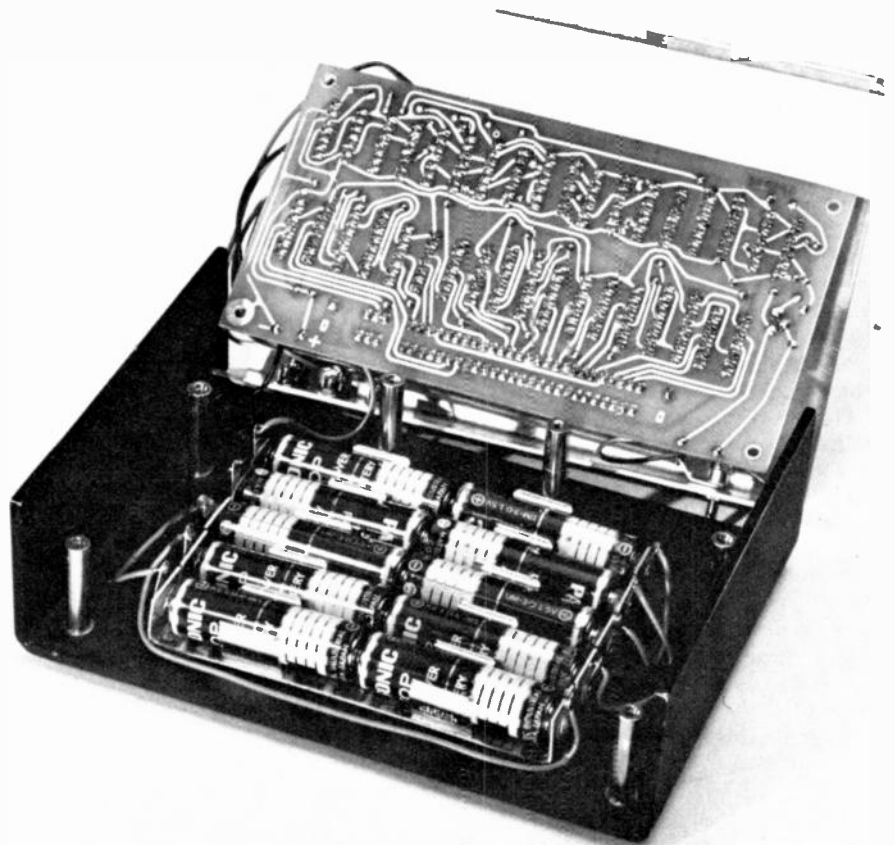
TEN PEN LIGHT CELLS IN BATTERY CLIPS, located under the circuit board, power this clock. As battery replacement is not frequent compact stacking is practical.
