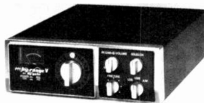
THE HY-RANGE V is a synthesizer AM/SSB rig whose circuitry is more complex.
