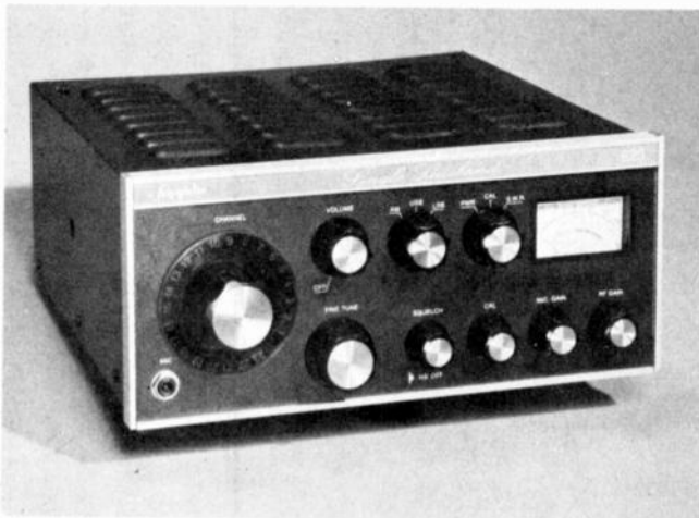
HY-GAIN 623 has features and looks of a ham-band transceiver.
