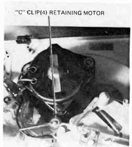
FIG. 6—C CLIPS hold the motor in place. Remove them, then the motor, to get at the upper motor bearings.
