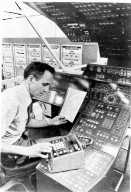
NASA ENGINEER T. D. JEFFCOAT punches a combination of load and power for a simulation run into the data entry panel in the cockpit test setup at NASA's Manned Spacecraft Center. The five consoles in the background simulate the electrical loads for the nose, electronics, air lock, intervehicular activity and tail compartments of a hypothetical space shuttle vehicle.
