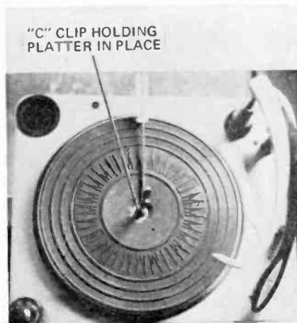
FIG. 1—TYPICAL RECORD CHANGER. Note that there is usually only a single C-clip holding the platter in place.
