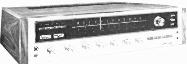
REALISTIC QTA-790 from Radio Shack (left above) is a 4-channel remote/preset stereo receiver. Favorite FM stations can be preset.
