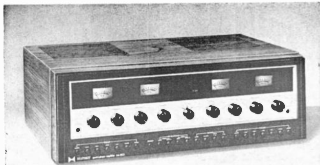
HEATHKIT AA-2010 (left) is a complete 4-channel integrated amplifier and preamp. It includes front-panel speaker switching.
