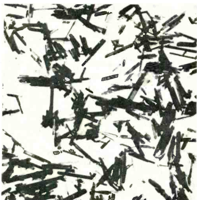
FIG. 1—(above) CHROMIUM-DIOXIDE TAPE has a denser oxide layer than conventional iron-oxide tape (FIG. 2, below). You can easily see the difference in these microphotographs.
