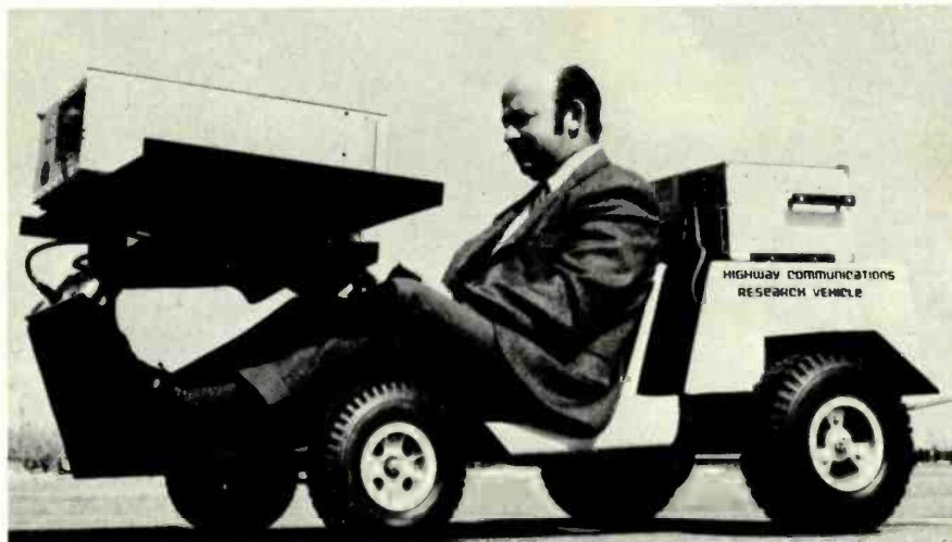
THIS RESEARCH VEHICLE was developed by GTE Sylvania to evaluate buried antenna models in a test roadway. It measures signal strength and noise levels. On the basis of test results, antenna models and related equipment and techniques will be recommended to the Federal Highway Administration for developing a highway communications system. R-E
