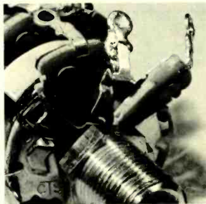
FIG. 4—KICKED BY A RIDER, this unit still worked—with one intermittent channel.
