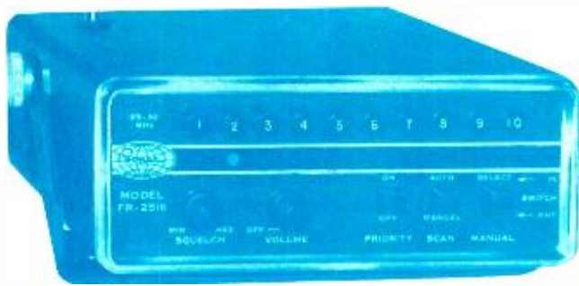
SONAR 10-CHANNEL LOW-BAND RECEIVER (above) scans 20 channels per second and samples priority channel every 2 seconds for 40 msec. Manual selection scans slower. PACE SCAN 202-HL (top right) tunes 8 channels between 25 and 512 MHz. The set, by Pathcom, has ceramic filters for good adjacent-channel rejection; 12-volt dc and 117-volt ac supplies. JOHNSON'S DUO-SCAN FM MONITOR (at right) covers 8 channels in 30-50- and 150-174-MHz bands. Receiver is double superhet and operates from 11-16 volts dc and 117 volts ac.
