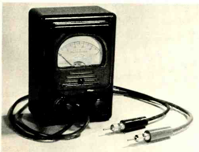
PHOTOGRAPHER'S TEST METER contains special circuitry ideally suited to in-the-field testing of photo gear. It's self-contained, and small enough to carry easily along with your normal photo gear.
