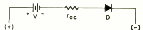
Fig. 6—EQUIVALENT CIRCUIT of a forward-biased diode. Diode D conducts when applied voltage exceeds battery V .
