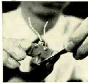
MOUNTED IN HEAT SINK, the tiny laser (at tip of the pointer) draws about 1.5 W.
