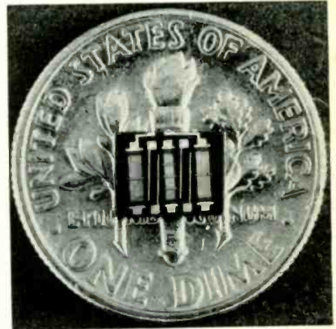
Three SWIF combs are combined into single unit shown in photo. Center comb, with about 20 fingers, serves as transmitter; two outer combs are series or parallel connected. Diagram above is of SWIF i.f. unit formed on a 2 x 1-inch substrate with IC amplifiers.
