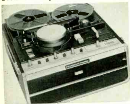
Compact vtr by Panasonic uses standard 1/2-inch tape, and can record NTSC color. Automatic-control circuit corrects phase and frequency fluctuations. It will be available this year.
