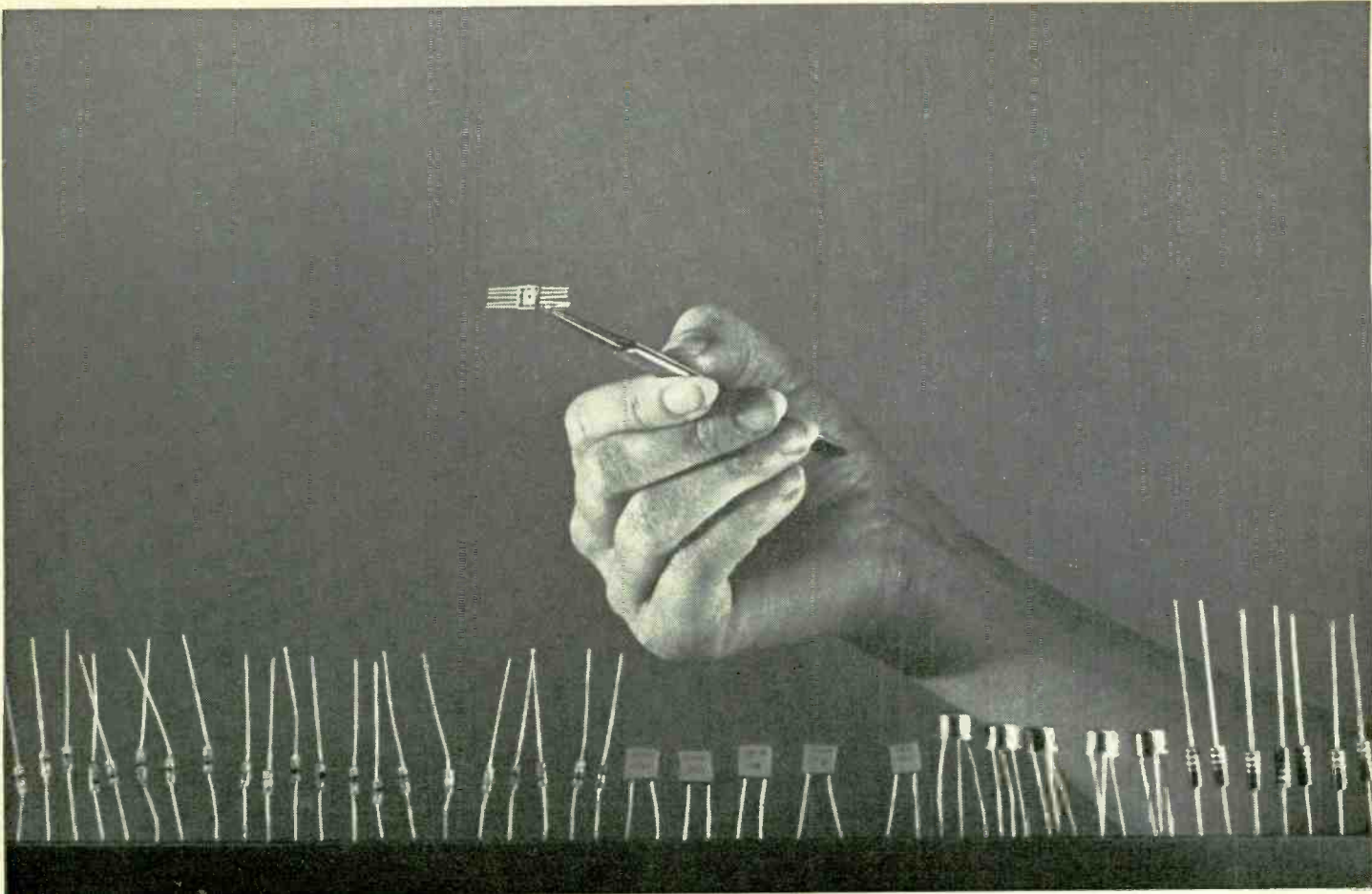
50 functions in a single chip. The functions of 50 separate transistors, diodes, resistors and capacitors can now be performed by the tiny dot in the center of the integrated circuit held by the tweezers.
