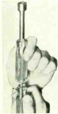
Fig. 10—Hole through the handle speeds locknut and control-shaft adjustments. Xcelite makes it.
