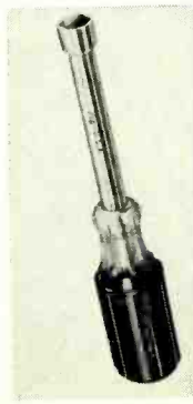
Fig. 6—Rubber handles on a nutdriver don't add insulation, but do add drive power by giving user a better grip. Klein model 630 shown.
