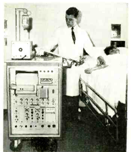
Fig. 2—Patient-monitoring systems like this one are saving many lives by spotting small but critical changes in patient life functions. System are modular.
