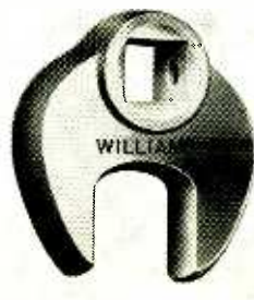
Fig. 23—Crowfoot adapter works like an open-end wrench. Extremely useful where you can't slip a socket over a bolt or nut. Unit shown is Williams model BC-1700.
