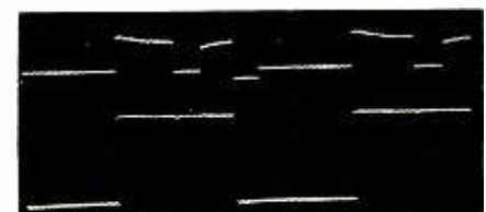
Photo B: Waveforms at G (top) and E. Frequency is 1 kHz, delay 500 \mu sec.
