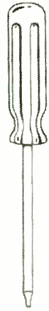
Fig. 6—Square-tipped screwdriver comes in five tip sizes. Unit shown here is Vaco driver model R10.
