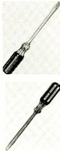
Fig. 17—Insulated-blade drivers, like the Crescent 2401-4 (left) or Klein 620 (right), have only the tip exposed, which simplifies working around dangerous voltages.
