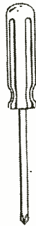
Fig. 4—Clutch-head or V-slot looks like a Phillips but isn't. Tool at the left is the Vaco model F-710 screwdriver.
