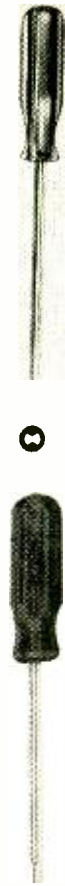
Fig. 5—G-type clutch-head is still another tip style. This time only two such screwdrivers are shown. Left, Xcelite 3164; right, Ocatonna CH 6.
