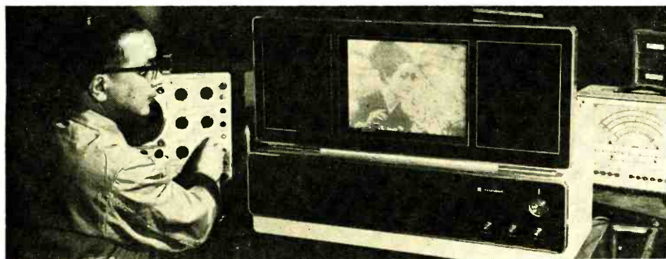
Experimental flat-screen set is checked by project director Yoshiyama. Model uses some 8600 components.
