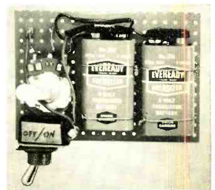
Simple perf-board mounting of two 9-volt batteries, switch and 1-megohm pot provides a variable bias source. The circuit for this setup is in Fig. 1 below.
