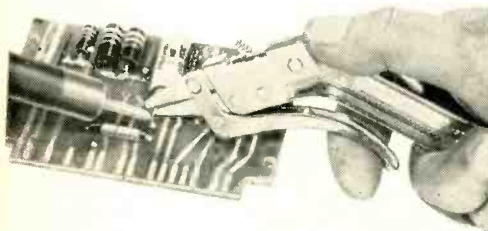
A "third hand" for small assembly work, the X-Acto Lock-Griplier also serves as a wrench, stripper, wire cutter and pliers.
