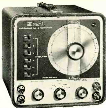
Knight KG-688 Sine/Square Wave Generator. Square wave function is useful.
