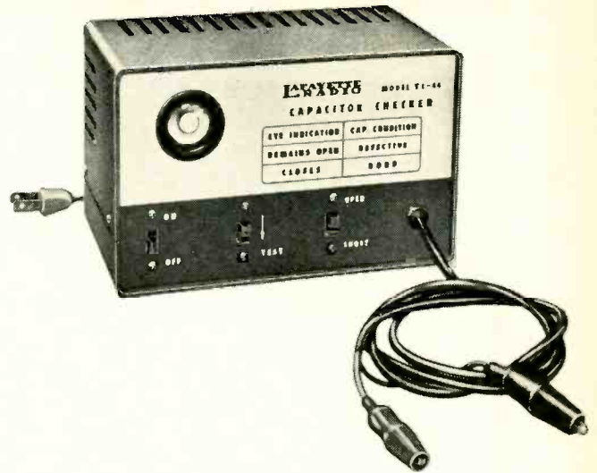
In-circuit capacitor tester (Lafayette's Model TE-44 above) uses electron-ray indicator. Checks values from 10 pF to 2000 pF. Sprague Model 2W1 meter shows capacitor values.
