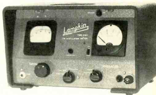
Peak frequency deviation on FM mobiles can be measured with Lampkin Type 205A. Tests signals in 25-500-MHz range.
