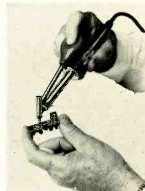
Self-adjusting wire stripper (top right) takes any wire from AWG No. 8 to AWG No. 24. Plastic grips. Telvac Model T-52.
