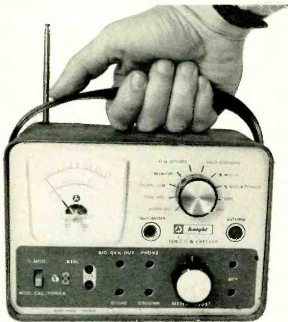
CB testers like this Knight (Allied) Ten-2 model combine several useful test functions in one portable cabinet.
