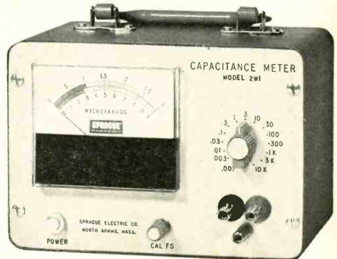
In-circuit capacitor tester (Lafayette's Model TE-44 above) uses electron-ray indicator. Checks values from 10 pF to 2000 pF. Sprague Model 2W1 meter shows capacitor values.
