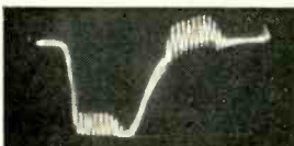
No back porch; color information on top of sync-pulse makes sync difficult on some sets.
