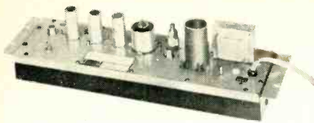
Example of a one-channel, or strip, uhf amplifier, the Blender-Tongue MCS-U.
