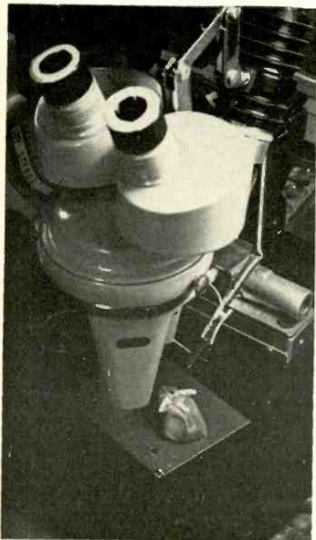
By attaching microelectrodes (left) to the bollworm's tympanum nerve, researchers determine its hearing-frequency range. Shown
