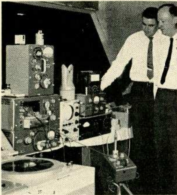
Quite an impressive table full of equipment is needed for professional measurement of reverberation. Permanent sound-system console at left is part of hall.
