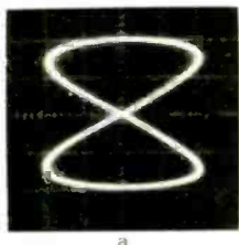
Fig. 6-a—This figure 8 shows proper pilot phase with respect to the subcarrier (see text). b—Composite output for either the R or L input only.
