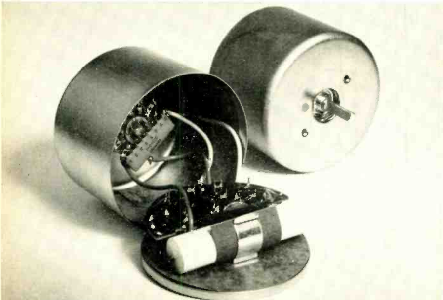
The Texas Instruments moisture-control module as used in automatic clothes dryers.
