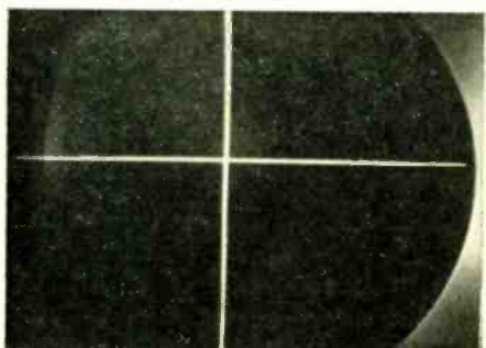
To set dynamic convergence, the single crosshatch is most useful on the CG-141.
