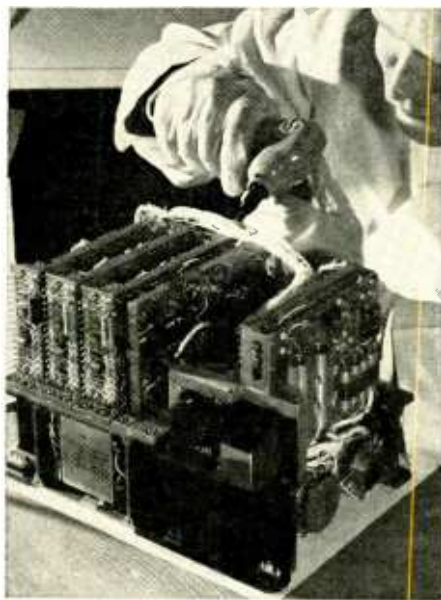
Containing over 1,500 components, this IRU device guided the Lunar Orbiter.
