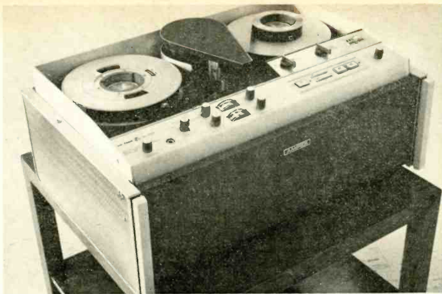
Ampex VR-7000-A can record and play back tapes in either color or black and white.
