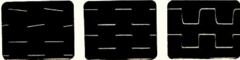
Fig. 4—Square waves through 30/30: left to right 20, 2,000, 20,000 Hz. Lower trace in each picture is input waveform. The output load is 8 ohms in each case.
