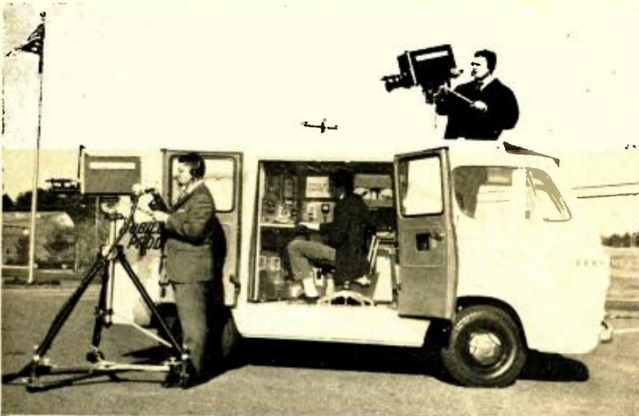
TV STUDIO CONTROL ROOM on wheels for use in educational television has been introduced by Sylvania. The 211-cubic-foot unit—an air-conditioned Chevy-Van—includes a power generator, video tape recorder, monitors, two TV cameras with viewfinders, tripods, dolly equipment, portable lighting unit and power and camera cable. One of the cameras can be elevated through a hatch in the roof for over-the-crowd shots.
