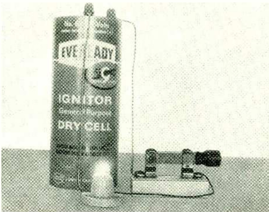
Simple circuit symbolizes basic principle of electric current flow between two points.
