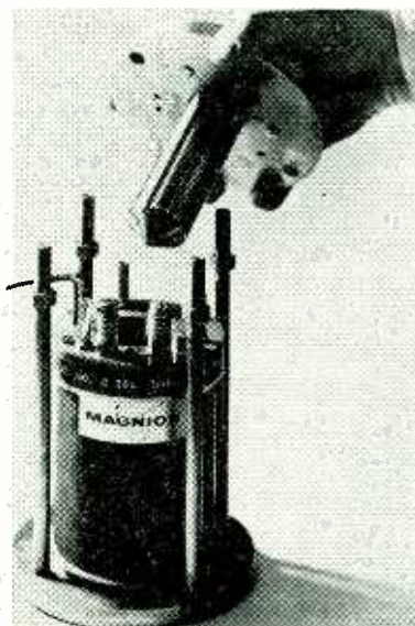
Magnet (top) becomes superconductive by immersion in liquid-helium tank (bottom).
