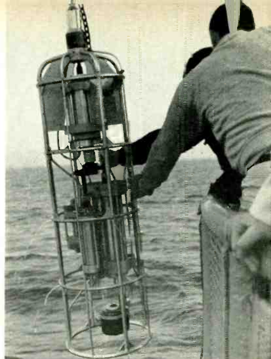
Instrument package used beneath the sea telemeters its measurements to surface by FM. Schematic (below) is transmitting circuit for measuring the salinity of the sea water.
