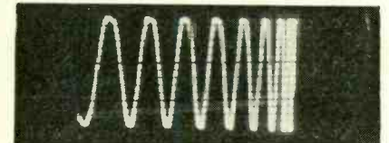
Fig. 4—This is horizontal nonlinearity, which shows up as crowding of the trace toward right of screen. Trouble could be in oscillator or horizontal amplifier.
