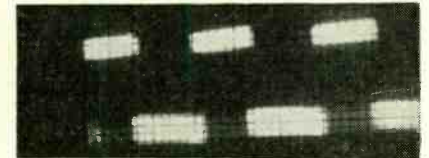
Fig. 3—Broad, blurred trace as in this square wave usually means hum in vertical amplifier. A 30-Hz sweep shows blur for what it is: 60-Hz jitter on trace.
