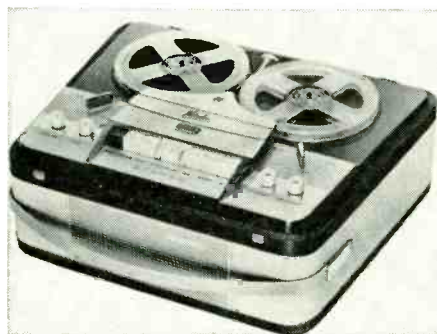
Norelco 401 is typical of medium-priced high-quality home tape recorders. Push-button control. 4-track stereo record and play, sound-on-sound recording, tape index counter (rear, between reels). Machine has four speeds: 7\frac{1}{2} , 3\frac{3}{4} , 1\frac{7}{8} and 15/16 ips.
