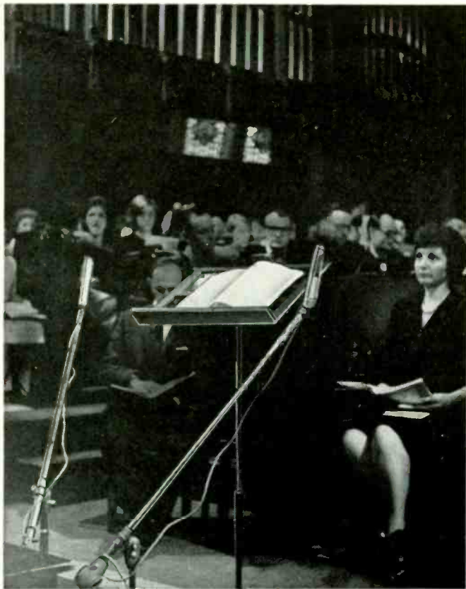
Two B & O bidirectional ribbon mikes were used for soloists in this church choir recording (stereo). Overall choir and organ pickup was left to two Synchron cardioid condenser mikes, suspended about 12 feet above the area in this photo. Two mikes might have been enough, but four gave an opportunity to experiment.
