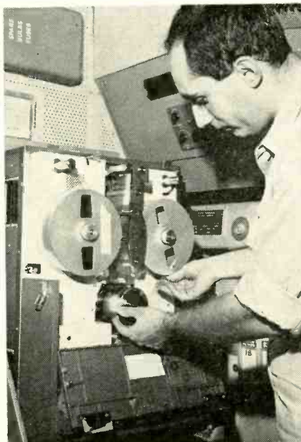
Technician changes tapes on the Sony Videocorder which supplies the closed-circuit TV pictures for American Airlines Astrovision. Beside the TV, stereophonic classical and popular music as well as live television and in-transit pictures of the terrain are furnished.
